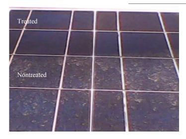
Solar panels treated with DSS nanotechnology coating:
